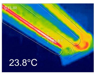
Highest temperature of an existing fluorescent fitting (left) and replacement LED fitting. (Infrared photos courtesy Tristram Buttner.)
